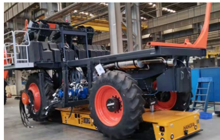
Cotton Picking Machine Transporter(40t)
