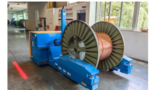
Customized Cable Transport AGV (8t)
