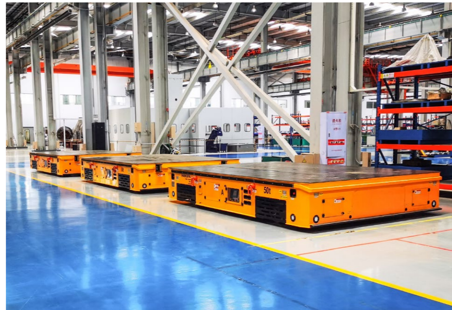
OmniRhino-Three-transporter Linkage Omnidirectional Transporters(50t x 3)
