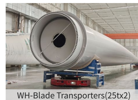
WH-Wind Turbine Blade Linkage Transporters(30tx2)
