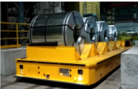
OmniTitan-Steel Coil Transporter(50t)
