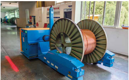
定制型拉线缆叉车AGV(8t)
